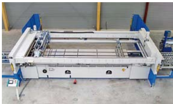
THE FLEISCHLE SH 1/2. AUTOMATIC SCREEN PRINTER FOR IN-LINE DECORATIVE PRINTING OF LARGE ARCHITECTURAL GLASS
